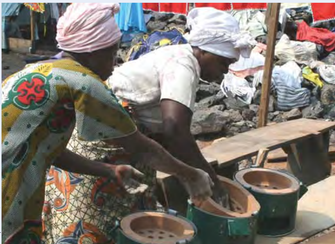
Members of a community cooperative build stoves that are energy efficient with tin and clay. Each stove will sell for between $5 and $9.
