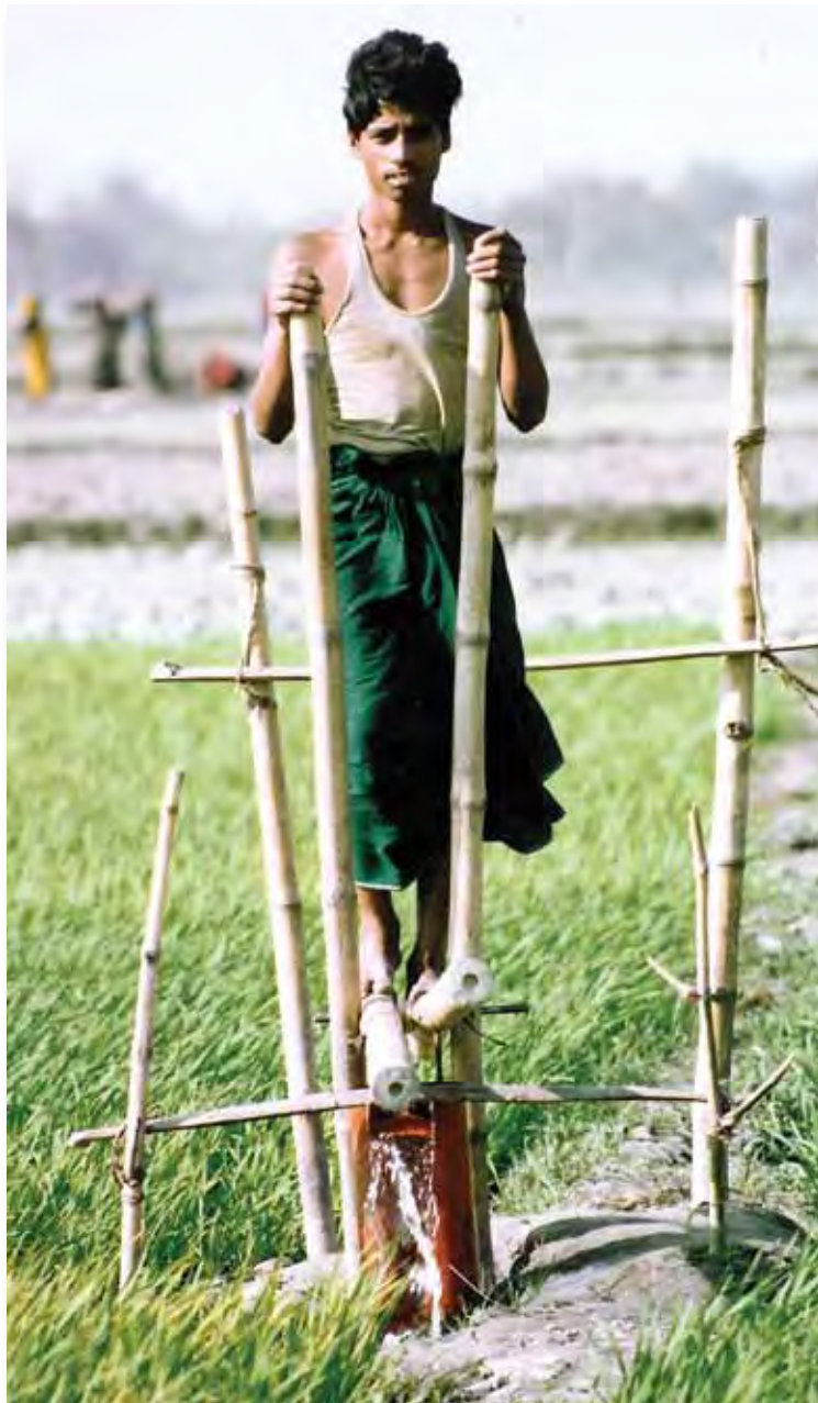
BAMBOO TREADLE PUMP Designer: Gunnar Barnes of Rangpur/Dinajpur Rural Service and International Development Enterprises, Nepal © 2002 International Development Enterprises
